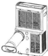
**Step 6:** Adjust the length of the flexible exhaust pipe and avoid bending it. Make sure it is near a power outlet.
