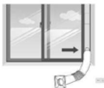
**Step 5:** Connect the hose connector to the output of the device.
