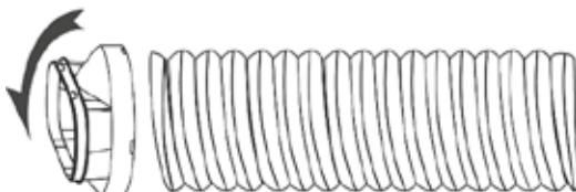
**Step 3:** Extend the adjustable window kit by the length of your window. Connect the air outlet tube to the window kit.
